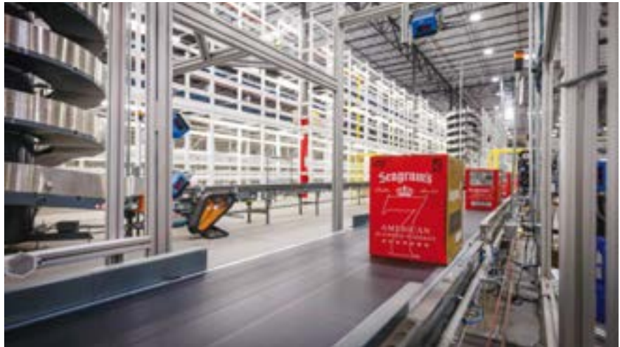
Cases are inducted and conveyed to the shuttle system.
